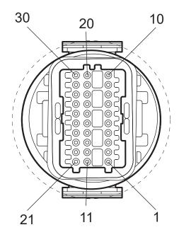
To enable the parallel connection, connect the data cable to pins 4 and 5 of the first inverter, which will become the **Master**, and to pins 1 and 2 of the second inverter, which will become the **Slave**. Repeat the same wiring procedure for all subsequent inverters.
