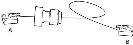
Connect the end of the cable with waterproof cover to the METER/CT port and the other end to the RJ45 extender, which serves as a connection between the communication line and the CT cable, as in the following diagram:
