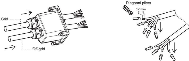
Prepare 2 penta-pole cables, then locate the European terminals and waterproof cover in the package. Connect the network cable to the GRID terminal block and any back-up line cable to the OFF-GRID terminal block. Connect the polarities of the lines to the terminal block in correspondence with the terminals, according to the order printed on the inverter casing. It is recommended to respect the cyclic sense of the phases. Reassemble the cover and tighten the cable glands.
