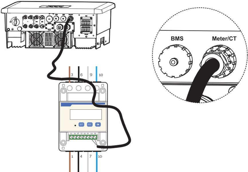
3. In order for the PSI-X-3PMETER-HY meter to work correctly, it is necessary to select the correct setting on the inverter; from the display go to the menu:
