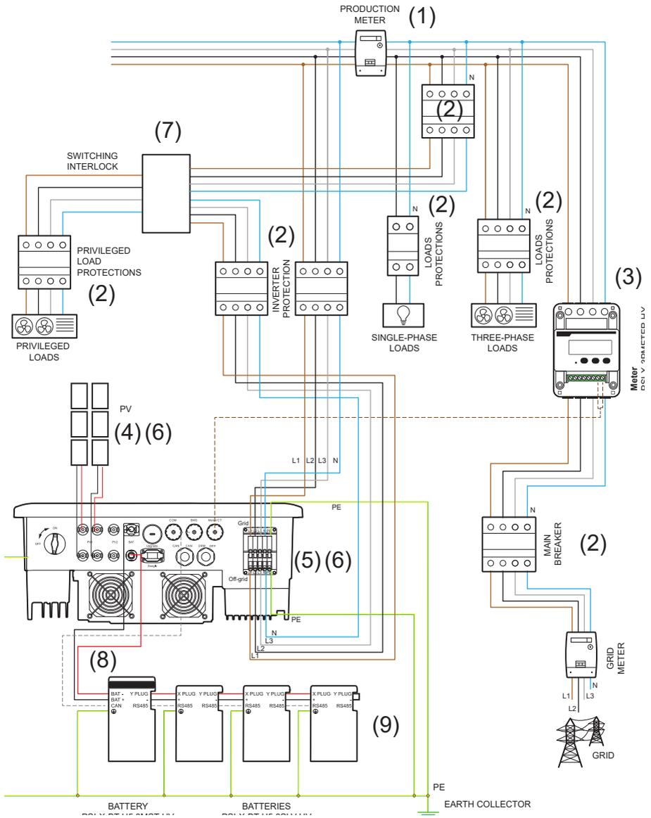
1. The position of the energy meter indicated in the diagram is purely indicative and to be evaluated in agreement with the project planner based on the regulations in force at the time of installation and of any other existing systems.
