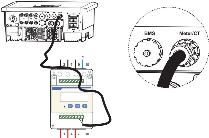
3. In order for the PSI-X-3PMETER-HY meter to function properly, it is necessary to select the correct setting on the inverter; from the display go to the menu:
