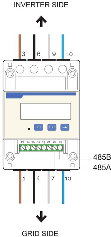
1. Strip the three phases arriving from the exchange meter (mains side) by 8-10 mm and attach them respectively to inputs 1, 4 and 7 of the meter by tightening the terminal.
