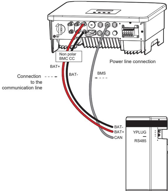
**Connection of PSI-X-BT-5.8SLV-HV batteries**
