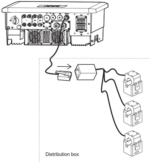
Check that the length of the entire line is sufficient to cover the distance between the inverter and the CT considering the length of the CT cable is 0.5 metres.
