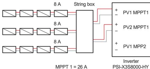
4. The strings can also be connected to both MPPTs (PV1 and PV2), through the use of a parallel panel.
