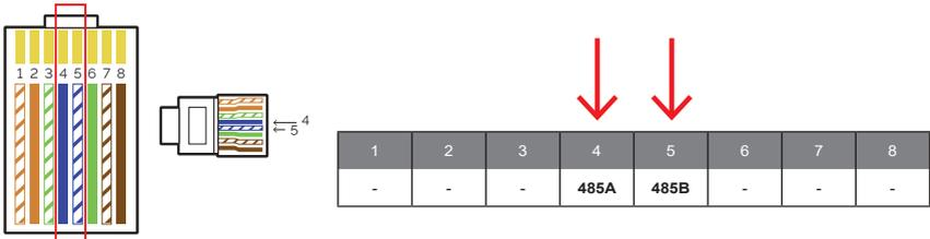
2. Connect the RJ45 plug to the Meter/CT port.
