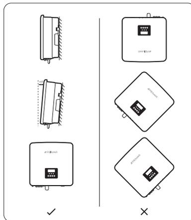
2. Install the inverter at eye level to facilitate viewing of the display and the possible maintenance activities.
