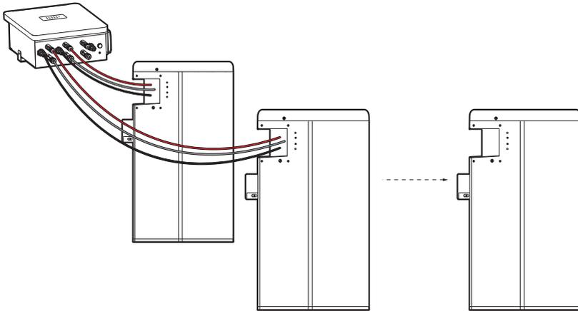
**Connection of PSI-X-BT-5.8SLV-HV batteries**
