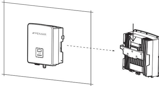
5. Use the TCEI wrench to tighten the internal hexagonal screw on the right side of the inverter with a tightening torque of  $1.2 \pm 0.1$  Nm
