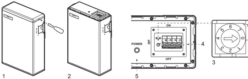
Start the battery only after turning on the inverter.
