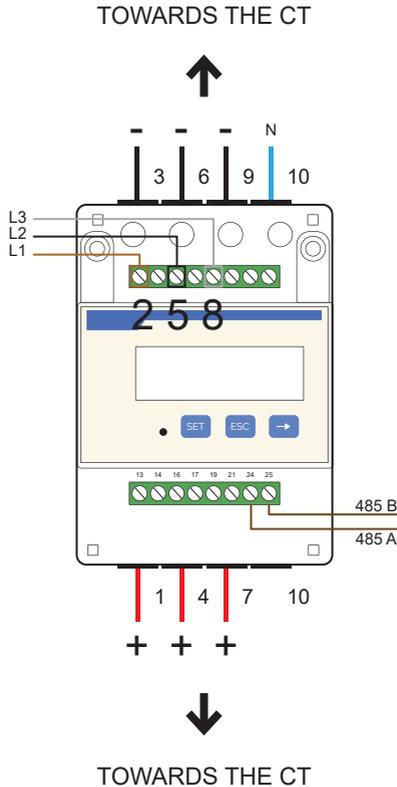
1. Create a derivation of the three phases arriving from the exchange meter, strip them 8-10mm and fix them respectively to inputs 2, 5 and 8 of the meter by tightening the terminal; the cable should have a section of 0.25~1 mm<sup>2</sup> (17~23AWG).
