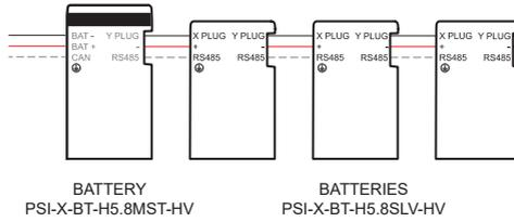
5. Insert the series termination wire into "-" and "YPLUG" on the right side of the last slave battery to complete the internal circuit.
